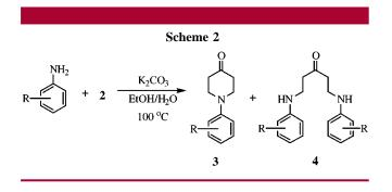
Utilizing this methodology, *N*-aryl-substituted 4-piperidones (Table 1) were obtained conveniently and rapidly in fair to excellent yields from a wide variety of anilines. The anilines
